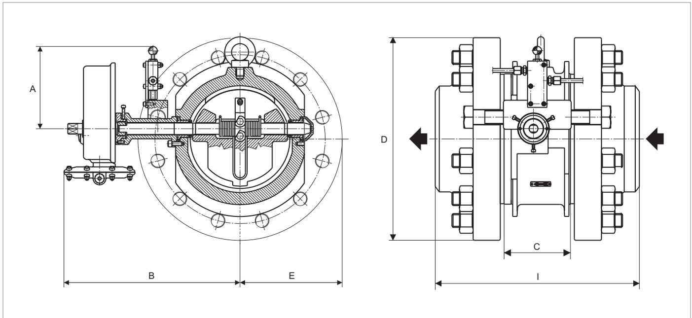
Figure 5. BM6X Series Dimensions
