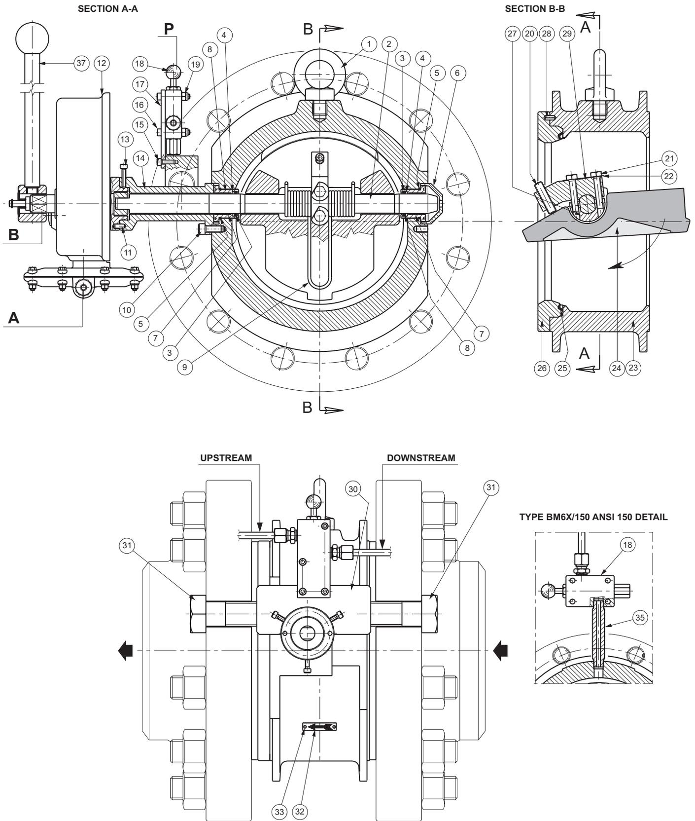
Figure 9. BM6X Series Slam-Shut Valve DN 80/100/150 Casting Version
