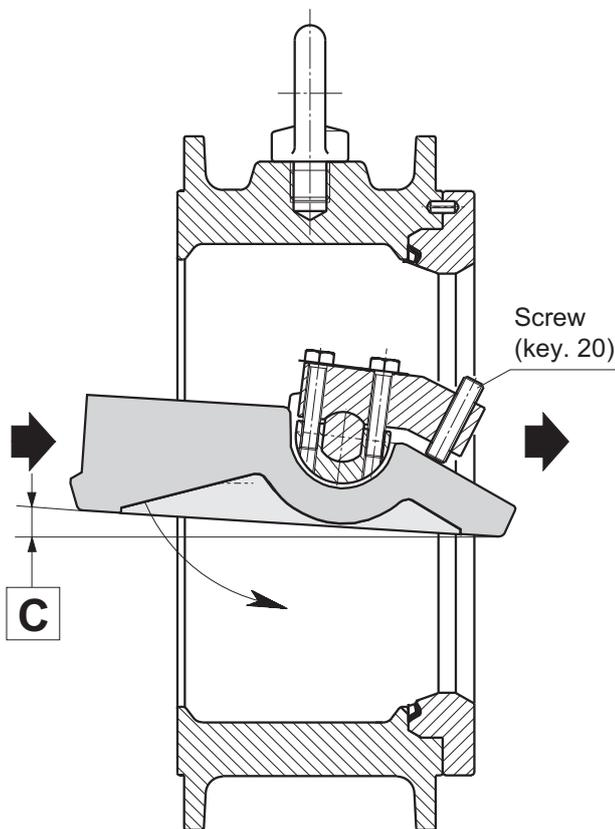
Figure 8. Type BM6X Shutter Position
